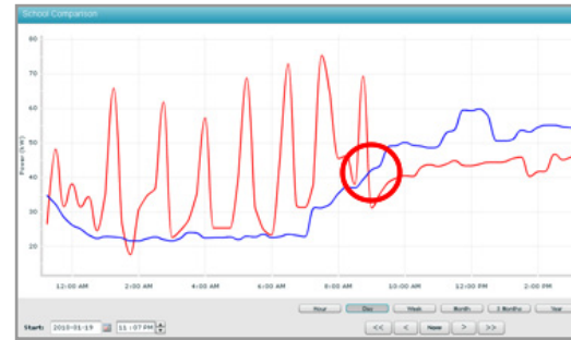
Figure 1 - The circled point highlights the exact time when Tahayghen Elementary’s boiler problem was corrected. Tahayghen Elementary’s energy consumption (represented by the red line) now mirrors a similar pattern to Dawson’s (the blue line).
